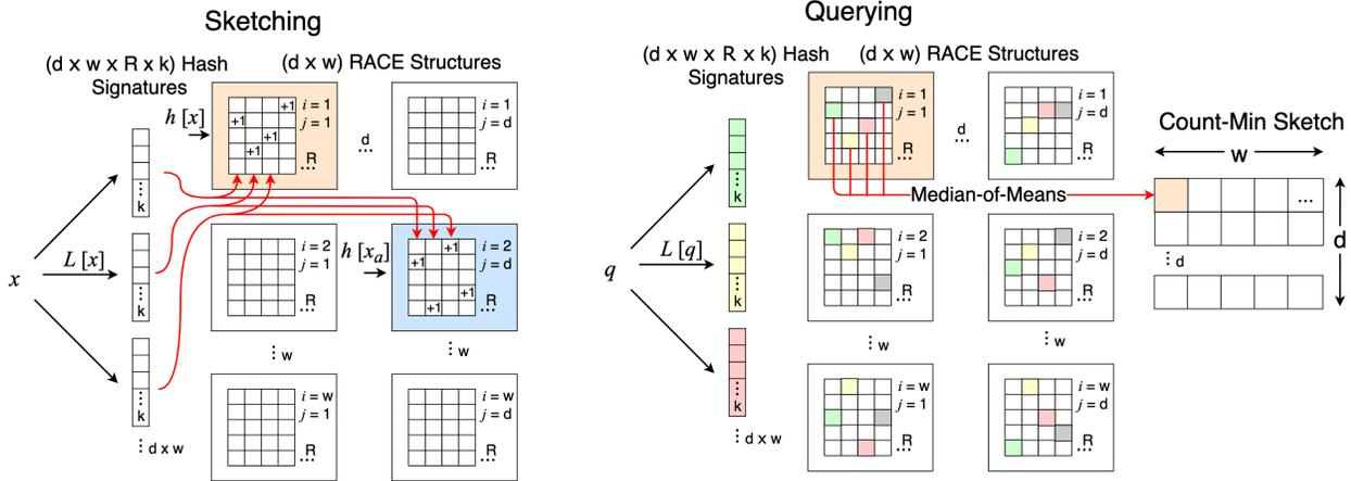
Figure 2. Implementation of sketching (Algorithm 1) and querying (Algorithm 2) using RACE data structures. During sketching, we compute  $d \times w \times R \times k$  hash values for each  $x \in \mathcal{D}$  and update the RACEs selected using  $h(\cdot)$ . During querying, we compute the hash values of the query  $q$  and estimate the CMS measurements.
