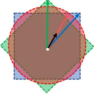
Figure 1: A depiction of the steepest descent directions for  $\ell_\infty$ ,  $\ell_2$ , and  $\ell_1$  norms. The gradient is the black arrow, and the  $\alpha$  radius step sizes and their corresponding steepest descent directions  $\ell_\infty$ ,  $\ell_2$ , and  $\ell_1$  are shown in blue, red, and green respectively.
