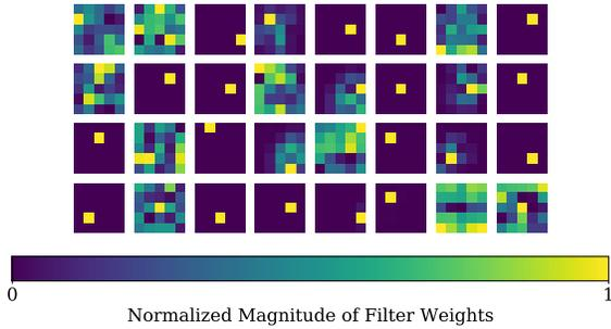
Figure 3: A view of each of the (5x5) learned filters of the first layer of a CNN robust to  $\ell_\infty$  attacks. The singular sharp values are characteristic features of models robust to  $\ell_\infty$  attacks.
