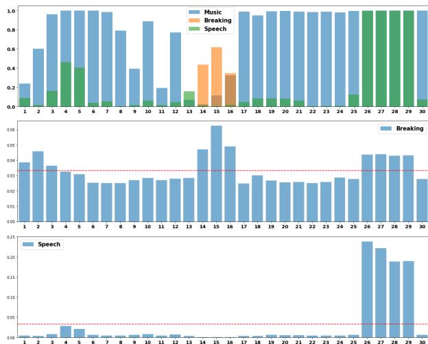
Figure 1. An example of WEANET outputs on a recording from test set. Top: Segment level probability outputs for three classes present in the recording. Mid: Segment wise attention weights ( \mathbf{A} ) for the Breaking Sound. Bottom: Segment wise attention weights ( \mathbf{A} ) for the Speech Sound. Red line denotes if all segments were given equal weights (1/30).
